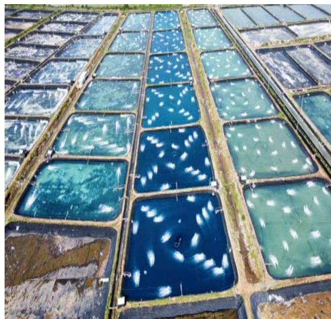
Figure 2. Positioning of aerators in groups creates zones where dissolved oxygen is concentrated. The number of paddlewheels (PW) is linked to pond carrying capacity; one PW is used to cover 100–150m 2 of pond bottom, every 25,000–35,000 post larvae or 400–500kg biomass.
