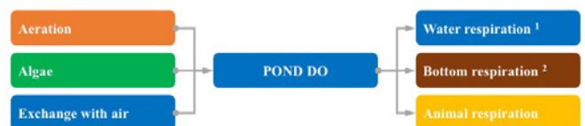
Figure 2. The main sources and consumptions of dissolved oxygen (DO) in a pond.
