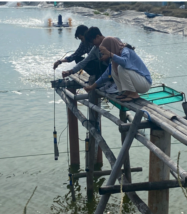
Aquaculturists in Singapore use three Aqua TROLL 500s to measure dissolved oxygen and other parameters to understand their water quality and adjust the level of aeration in their pond.
