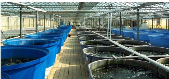
Tiltech Tilapia farm in the USA. A closed RAS under glass due to the cold winter temperatures.
