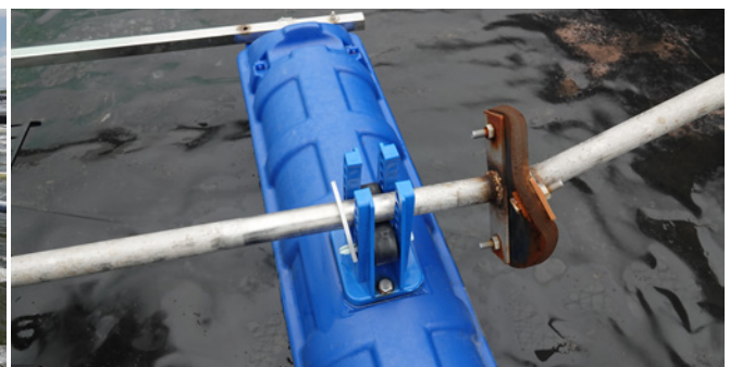
Energy optimisation is to explore the best aeration practice (left) and a roller bar is used to reduce friction during energy transfer via metal pipe to propel paddle wheel (right).
