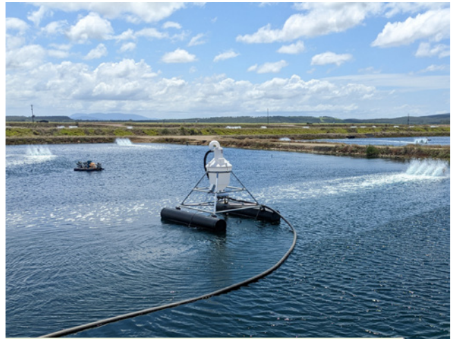
AQ1 Autofeeders operating at a farm. Picture credit: AQ1.
