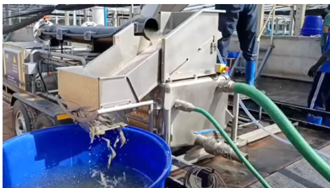
In-water shrimp stunner in operation in Asia. Photo credit: Shrimp Welfare Project.
