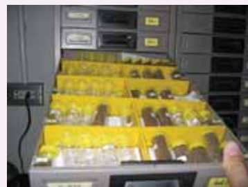
Feed samples are stored for three months in the quality control lab.
