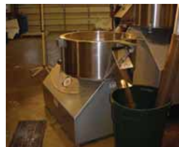
Micro-aquatic feed pellets discharging Spherizer
