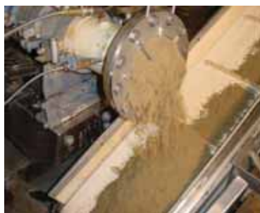
Wet strands of micro-aquatic feed diet coming from extruder and before Spherizer
