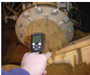
Measuring temperature of product coming from extruder
