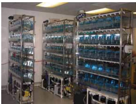
Aqua Bounty's two closed, recirculating, bioassay facilities where existing therapeutic products and new products under development are evaluated using live shrimp challenged with WSSV and other virulent shrimp diseases.
