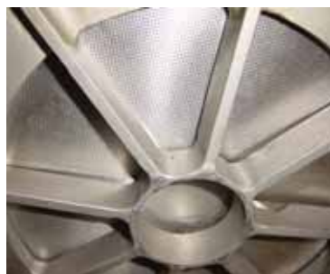
Close-up of extruder die used for forming wet strands of micro-aquatic diets
