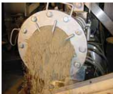
Wet strands of micro-aquatic feed diet coming from extruder and before Spherizer
