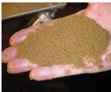
Micro-aquatic pellets after Spherizer and before drying
