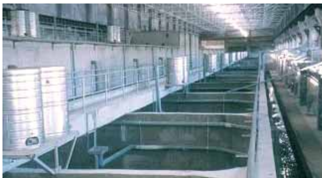
Hyper-intensive recirculating system designed and built for commercial production of grass prawn and other shrimp species
