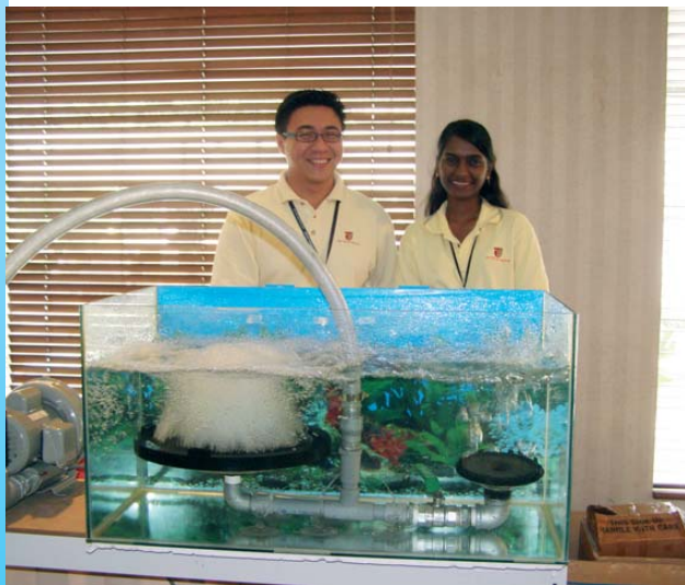
Rogini and Jimmy Cheong with a demonstration model of the diffusers in a tank with ring blower.
