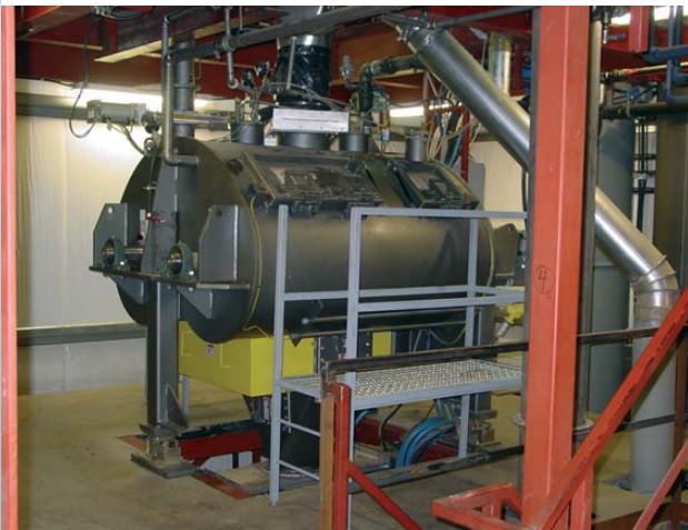
A Phlauer 2000L vacuum coater. A good vacuum coater manufacturer will ask the proper questions with respect to the number of liquids to be added and size the equipment properly to allow for a number of liquid additions either under vacuum or atmospherically (or both in one batch cycle) while maintaining the required production level. Picture courtesy of A&J Mixing, Canada.
