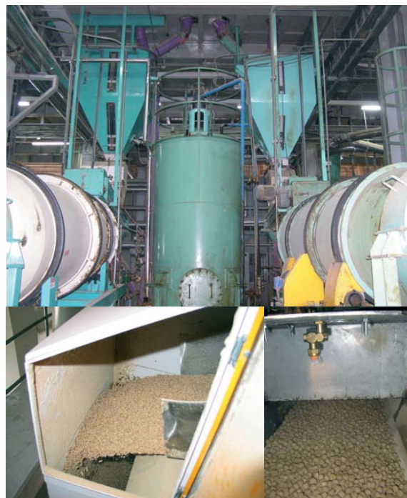
PPLA technology in the mill: Two feed producing lines equipped with surge bins, enzyme applicators and downstream fat coaters (top). The feed flow to the spray chamber is regulated to create a stable feed curtain (bottom left) onto which the enzymes are sprayed (bottom right).
