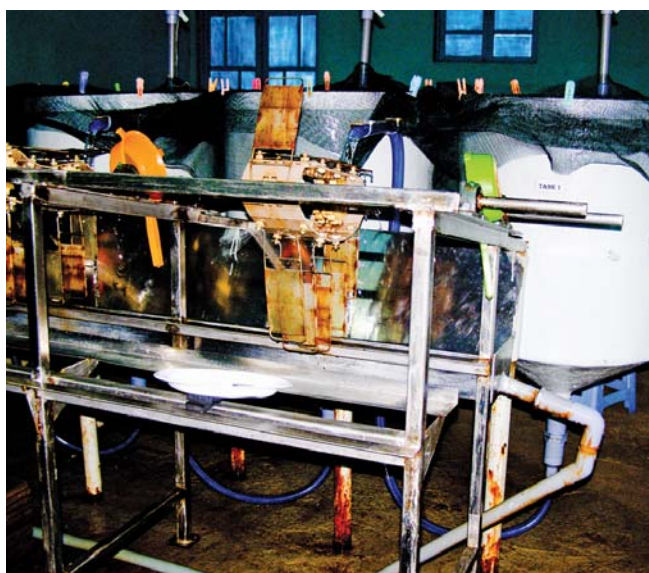
The automatic faecal collection system developed by INRA, France and the University of Laval, Quebec, Canada. In this system, water outflow from the aquarium is filtered continuously through metal sieves. The faeces are thus extracted very rapidly from the water (between 6 and 15 seconds after emission) and preventing their disintegration. The sieves transfer the faeces to a collection tank where they are immediately chilled and freeze-dried. The rate of recovery reached 99.6%. Initially designed for the rainbow trout, this apparatus can also be used for the Atlantic salmon, bass, eel, carp, koi carp, cod, catfish and tilapia. (INRA press service).
