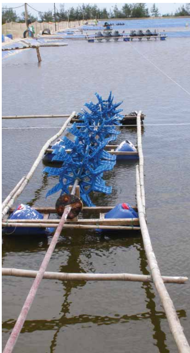
Le Mai with an aerator fabricated onsite using plastic piping. These aerators will disperse water upwards and long arm paddle wheels (left) will move water around the ponds.
