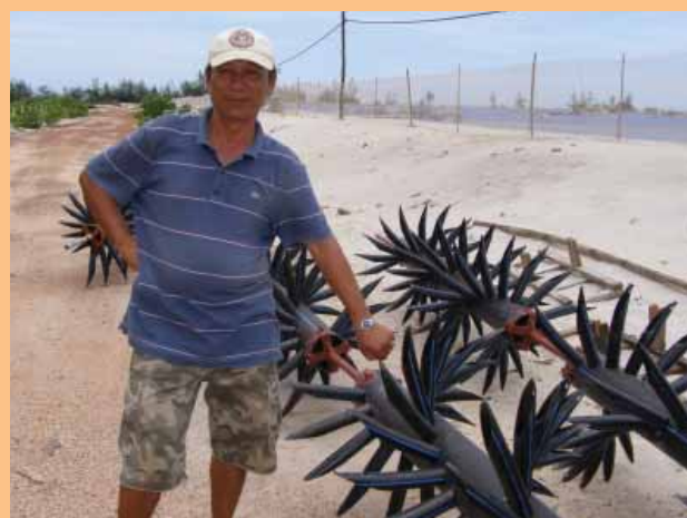
Le Mai with an aerator fabricated onsite using plastic piping. These aerators will disperse water upwards and long arm paddle wheels (left) will move water around the ponds.
