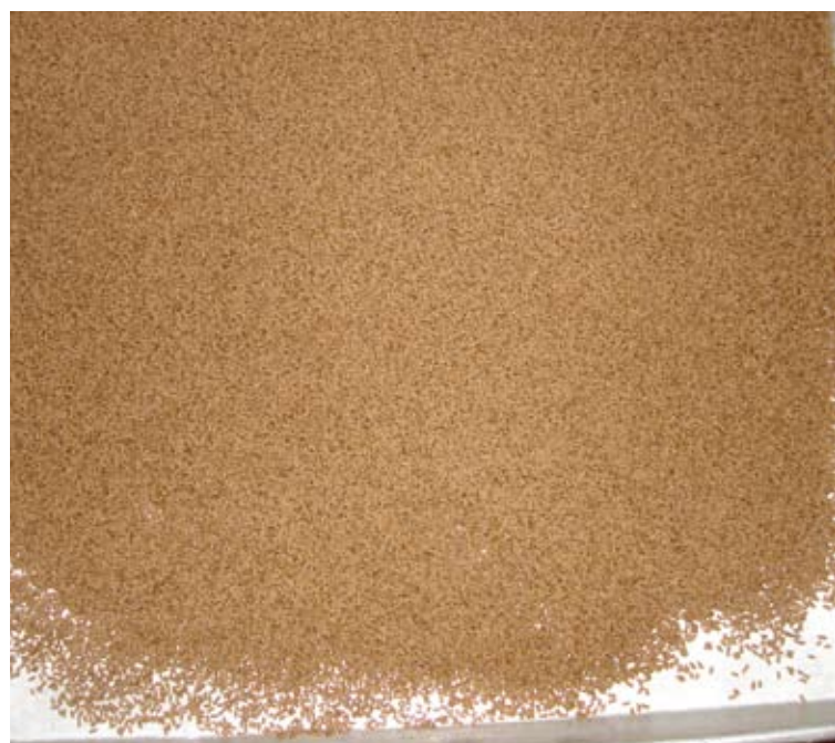
Photo of the typical evenness of a 1.5mm shrimp feed produced with the new technology.
