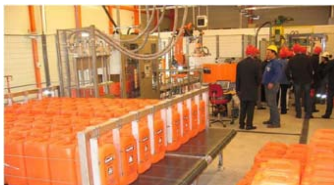
Liquid filling station for canisters
