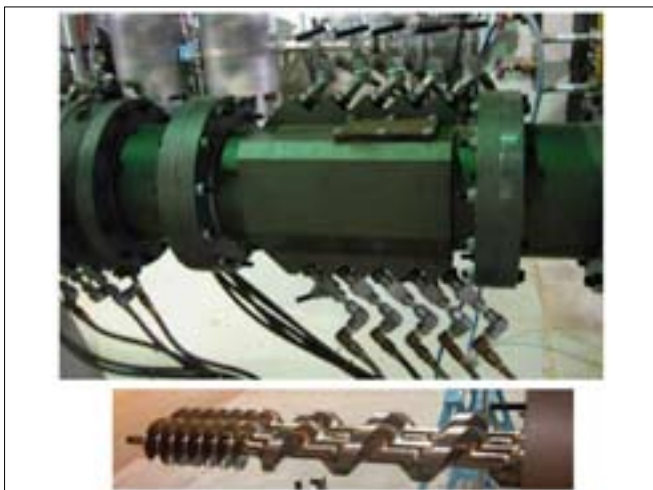
New thermal twin screw extruder
