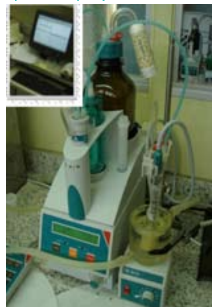
Figure 2. Automatic titrator precisely monitors feed protein digestion by species-specific shrimp enzymes.
