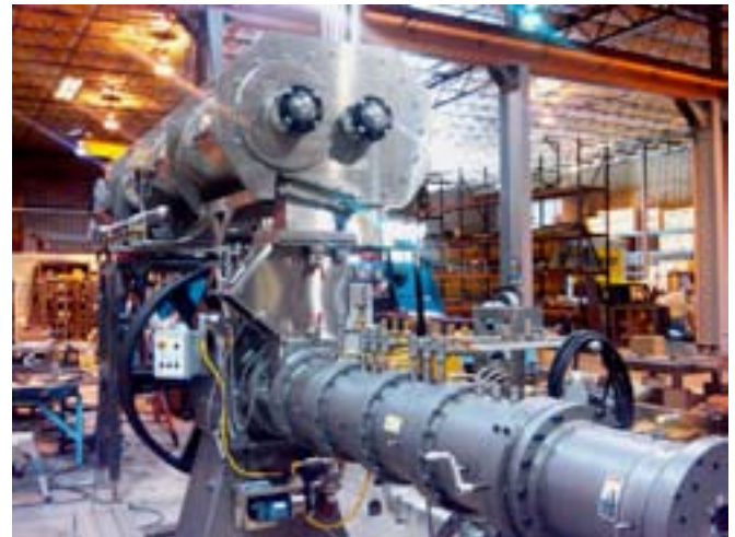
New single screw extruder with high intensity preconditioner
