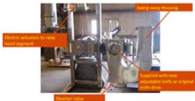
The new hygienic pneumatic pickup hood
