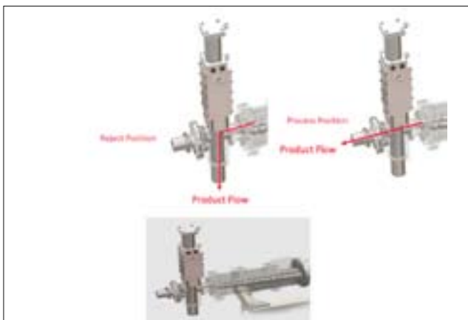
Back pressure valve in different position during extrusion
