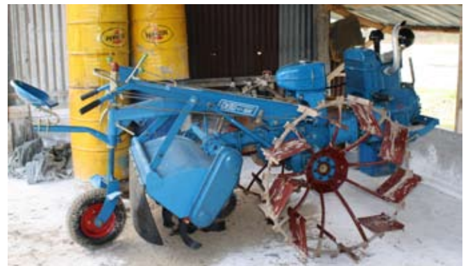
This is the innovative tiller for the ponds which Lim built in Malaysia using engine parts imported from China. With this, the soil preparation time is reduced and the ponds are cleaned well.
