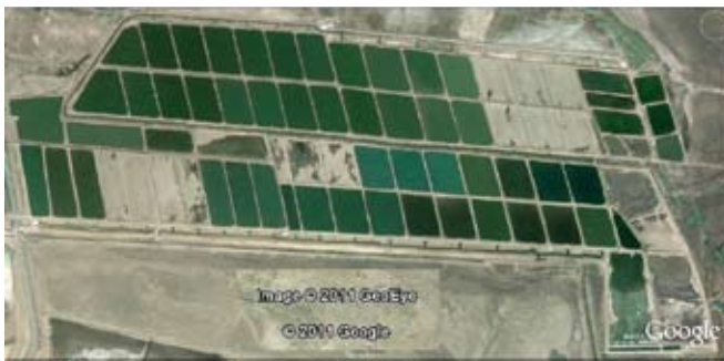
A well constructed farm in Surat showing settlement, reservoir and culture ponds with 5:20:75 ratio
