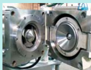
Extruder with Flextex installed
