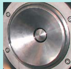
Venturi 100% restricted (small open area)
