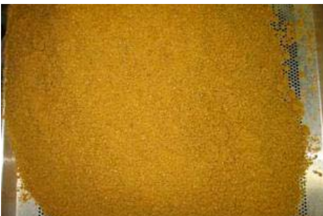
Photo 3. Material from HIP Preconditioner, 50% fresh meat, 11.5% steam, 3.4% water total of 35% moisture.
