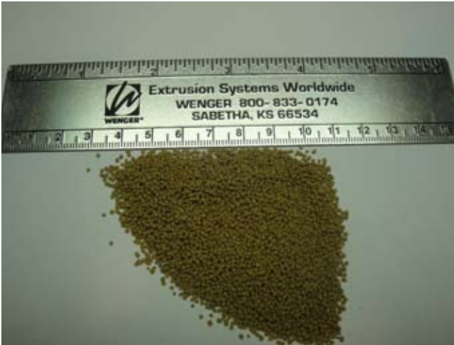
Photo 1. Shrimp feed through a 0.8 mm die hole. Single screw extruder.
