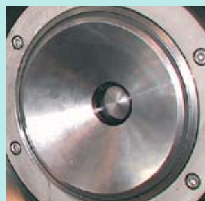
Venturi 0% restricted (large open area)
