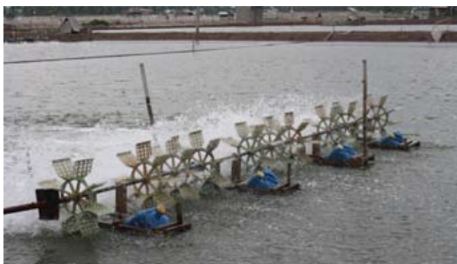
Long arm paddlewheels are the main aeration devices
