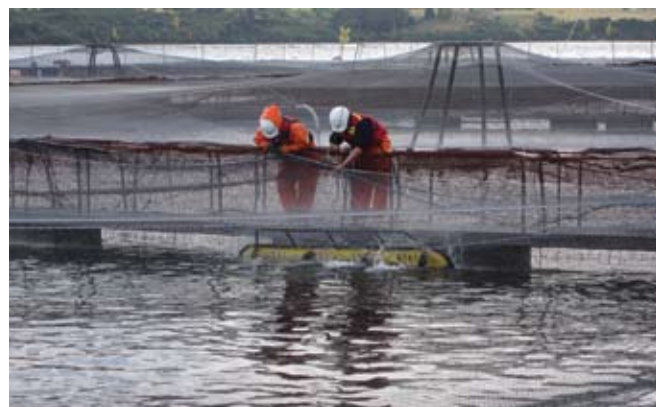
Operators monitoring the Terminator 9 net cleaner in use.
