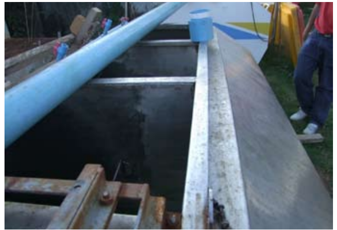
Transfer container with partitions
