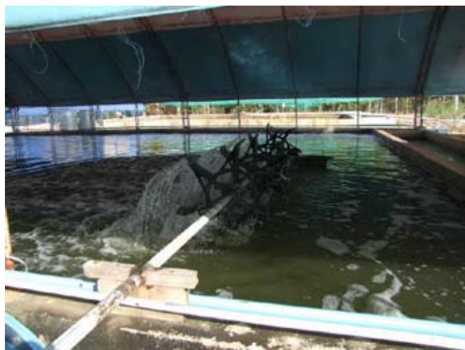
One long arm aerator in cement ponds.
