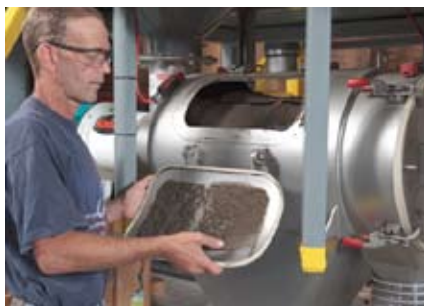
Inspection port allows operator to determine if screen requires cleaning.
