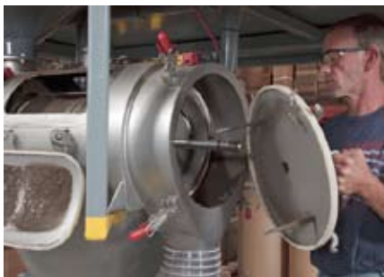
Hinged cover at discharge end of sifter allows cylindrical screen to slide freely from the cantilevered shaft for cleaning.
