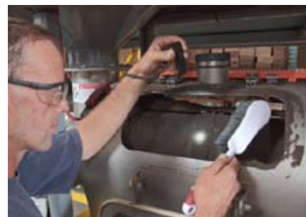
Inspection port allows operator to determine if screen requires cleaning.
