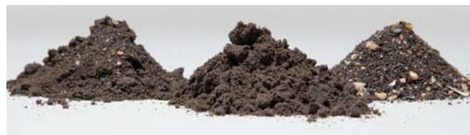
(L-R) Aquaculture feed product, screened product, and discharged oversize particles.
