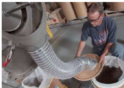
Oversize and agglomerated particles fill a container beneath sifter's discharge.
