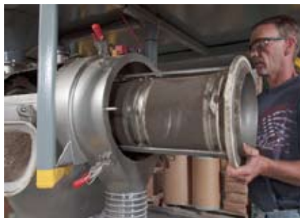
Hinged cover at discharge end of sifter allows cylindrical screen to slide freely from the cantilevered shaft for cleaning.
