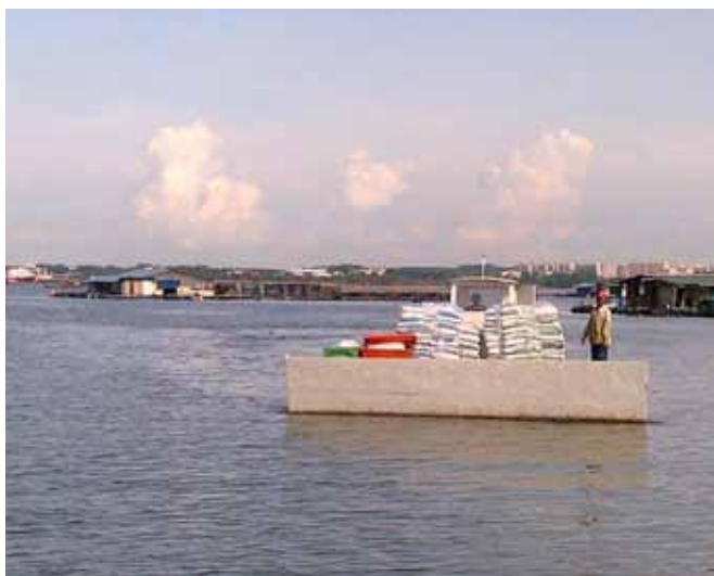
Workboat-5 transporting 12 tonnes of pellet feeds from the wharf to net-cages
