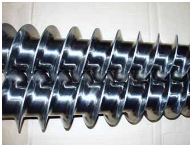
Conical co rotating twin screw design
