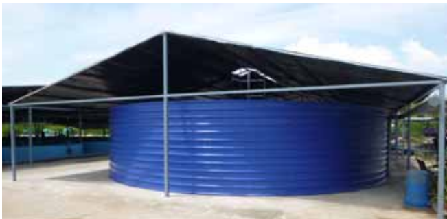
High wall and large 120 tonnes FRP tanks with nano-sterilization and degasser tower for larval rearing
