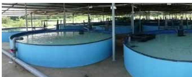
The new nursery area consists 20 units of 20 tonnes FRP (fibreglass reinforced plastics) tanks for nursing of seabass fry till 12g
