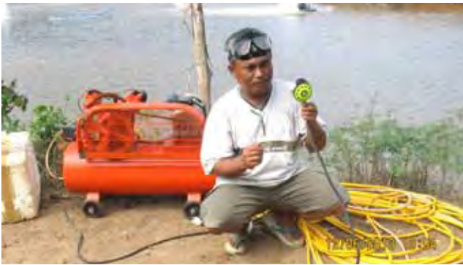
Technician Meryanto showing compressed air with breathing tool used in siphoning in Sumbawa Indonesia. Some workers can work under water and siphon up to 2 hours without surfacing
