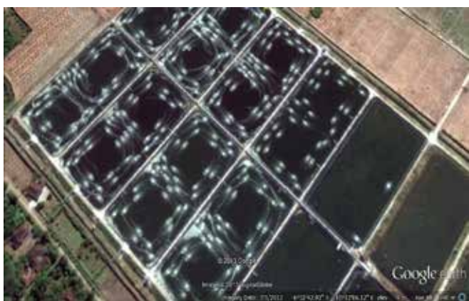
Google Earth image to show arrangement of paddlewheels in a long pond
