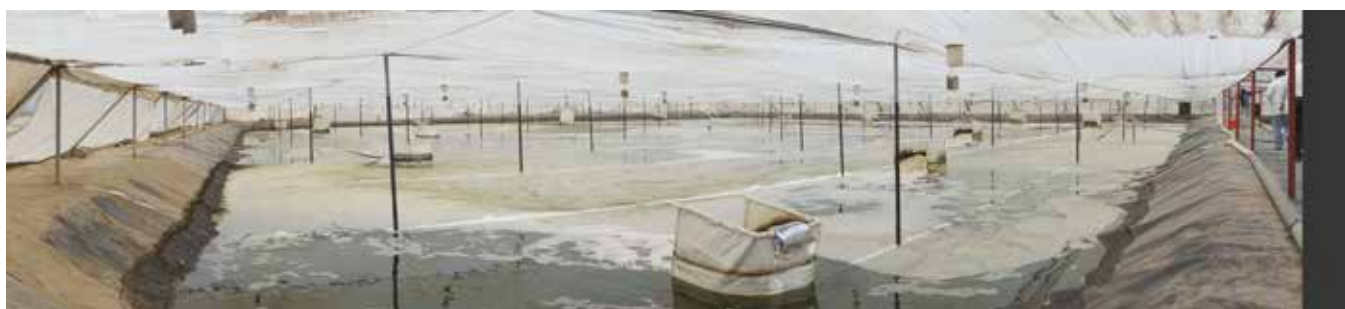
View of a hyperintensive pond with airlift units to aerate and produce water currents within the pond
