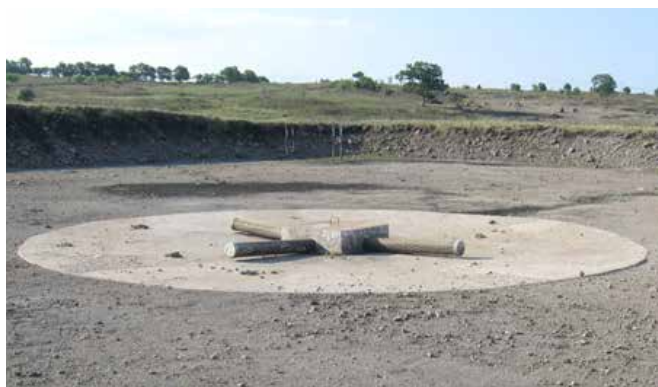
One example of a central sludge discharge system widely used in Sumbawa in Indonesia
