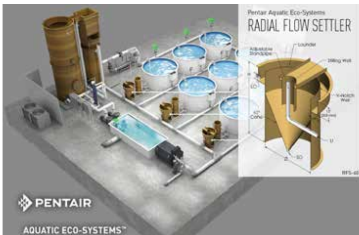
Diagram of radial flow settlers. Effluent water enters the RFS Liquid Inlet, flows upward through the adjustable Standpipe Assembly, and back down through the Stilling Well. Solid particulates settle to the cone bottom for removal through a Solids Outlet. The filtered water flows upwards over a V-Notch Weir into the launder, exiting through the Liquid Outlet.
