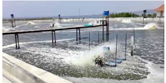
Blowers and paddlewheels vigorously aerate and move pond water.
