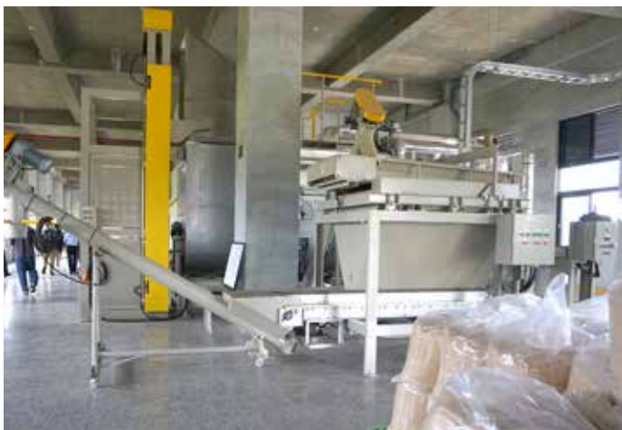
The BULK system includes a fermentation process of 6 hours at 70-75°C, drying and extruder for pellets with 10% moisture.
