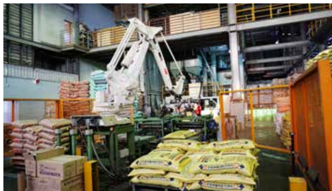
Automation at the factory with a robotic bag stacker
