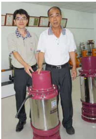
San Szu Chang (right) and son Evan Chang with the best selling BL1075C with an 8-inch pipe for a water flow of 7.5m 3 /min.
