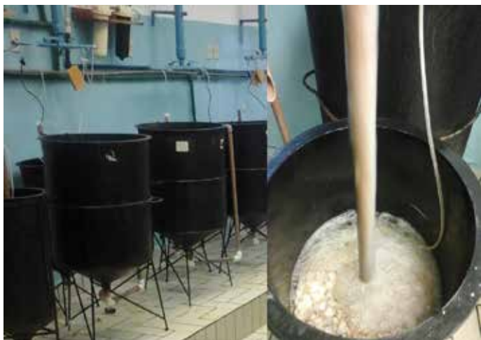
Figure 1. Example of closed system developed at CAUNESP-UNESP. The picture on the right shows the biological filter in use. The picture on the left displays the system as a whole.
