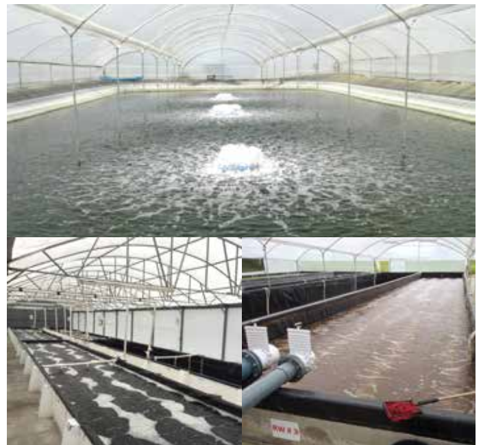
Rectangular tanks are easy to build, are space-efficient under standard greenhouses and familiarity of use by hatchery technicians.
