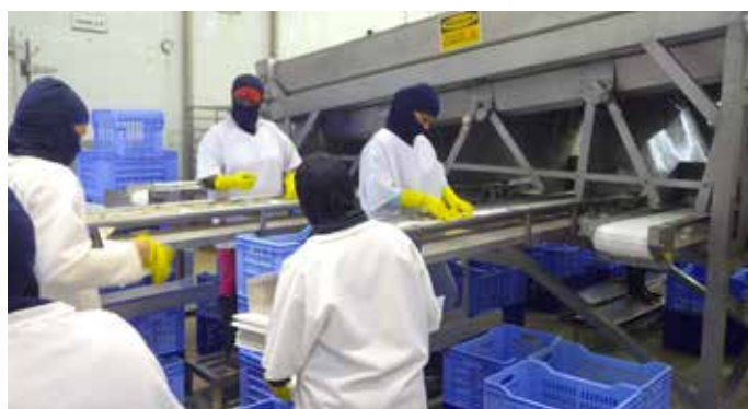
Inspection on lateral packing belts
