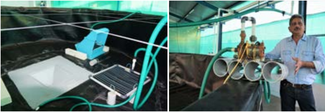
Anil explaining his latest venturi aeration innovation. Used in the larger N2 phase tanks, three sets of these four-tube venturi system pushes water at high speeds creating fine bubbles (right). This is an improvement over an earlier model used in the smaller N1 phase tanks (left, in blue). Next to this is the square device positioned over the discharge drain with the aero tubes to provide aeration from the bottom of the tank. Both these aeration devices are weighed down at the bottom of tanks.
