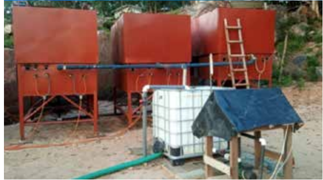
A treatment unit set on the shores of the lake to handle as many fry as possible. Top: one of the four circular tanks for treatment. Bottom: reservoirs of hot water delivered by gravity to the treatment tanks.
