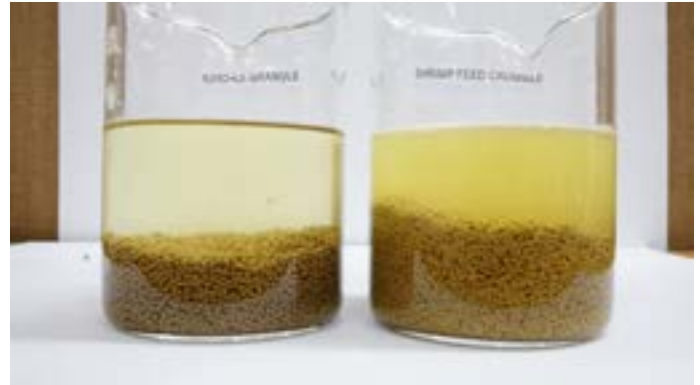
Water stability test. Extruded starter feed size 2B (1.2 mm – 1.6 mm, late starter feeds, left), do not leach as much as shrimp crumbles (right) after 30 minutes
