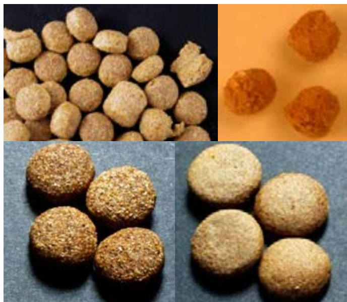
Figure 1. Four Photo Collection, First 3 cause fines in bag. 1st incorrect knife adjustment (top, left), 2nd wrong running conditions (top right) and 3rd coarse grind (bottom left), all cause fines development. 4th good grind and cut, reduced fines (bottom, right)
