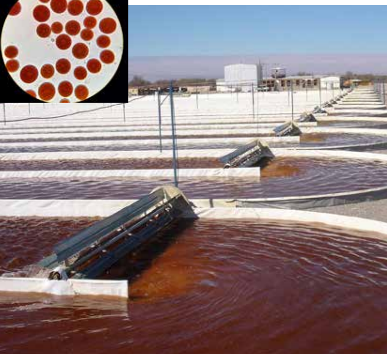
Production of natural astaxanthin Haematococcus pluvialis in raceways in Atacama Desert, Chile. Photo by Atacama BioNatural Products SA.
